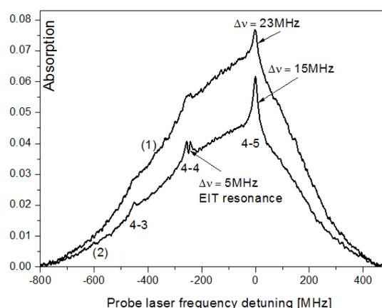
**Figure 2.** EIT and Dicke resonances at  $L = 1.5\lambda$ : (1) the probe laser is scanned within the  $F_g = 4$  set of transitions, no pump; (2) the pump laser is fixed at the 3 - 4 transition and the probe is scanned as in (1);  $T = 105$  °C, i.e. atomic density  $\sim 2 \times 10^{13}$  at/cm<sup>3</sup>,  $W_{\text{probe}} = 0.3$  mW/cm<sup>2</sup>,  $W_{\text{pump}} = 35.4$  mW/cm<sup>2</sup>.
