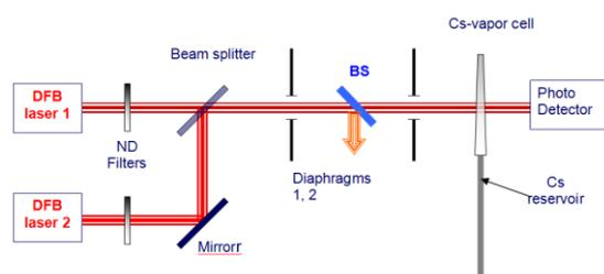
**Figure 1.** Experimental setup for VSOP, EIT and VSE resonance observation by pump-probe spectroscopy.
