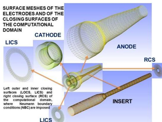
**Figure 2.** Surface meshes representing the electrodes of a coaxial gyrotron (2 MW/170 GHz) simulated by GYREOSS.
