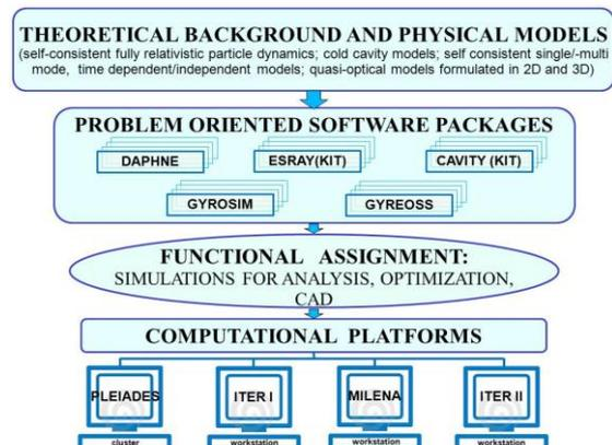
**Figure 1.** Structure of the simulation tools and computational infrastructure for numerical studies and CAD of gyrotrons.
