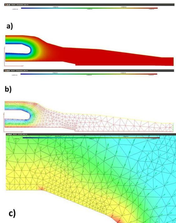
**Figure 3.** Electrostatic potential distribution (a); equipotential lines over the mesh (b); map and a vector representation of the electrostatic field near the emitting ring of the cathode (c), in a meridional cross-section of a coaxial magnetron injection gun (MIG) of the studied 2 MW/170 GHz gyrotron.
