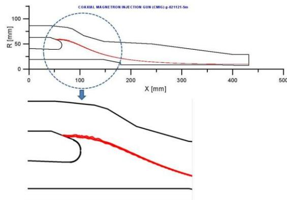
**Figure 4.** Geometry of the coaxial magnetron injection gun (CMIG) of a 2 MW/170 GHz gyrotron (black color) and electron rays (red color), traced by the novel relativistic particle pusher of the GYREOSS package.
